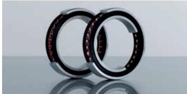
The reciprocal of bearing elasticity is stiffness. Stiffness indicates the resisting force of a preloaded bearing in newtons over its spring deflection in  $\mu\text{m}$ . Preload and stiffness are interdependent. As a rule, the stiffness of a bearing does not increase in a linear fashion in relationship to the preload. The axial and radial stiffness of a pair of angular contact ball bearings depends both on the preload and the contact angle.
