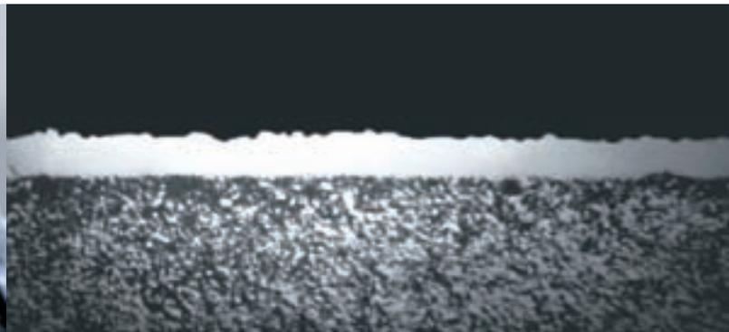
Fig. 10.2: Cross-section of ATCoat coating
