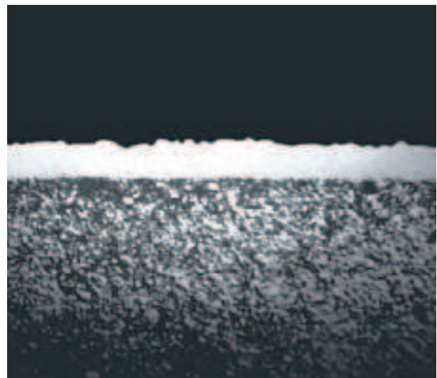
Fig. 8.2: Cross section of the ATCoat coating
